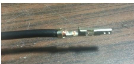
6. Add a little bit of solder to the connector to ensure it will hold forever. After that you can use this crimp in the expansion connector.
