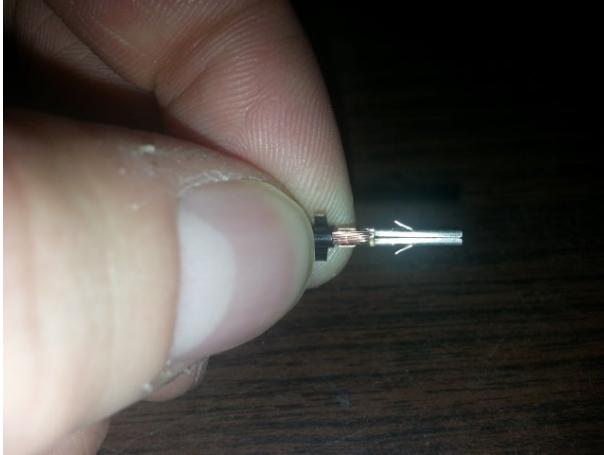
3. With long-nose pliers fold the small edges.
