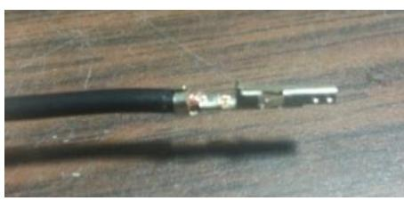
6. Add a little bit of solder to the connector to ensure it will hold forever. After that you can use this crimp in the expansion connector.
