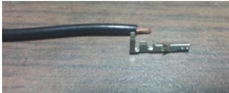
2. Insert the wire into the connector:
